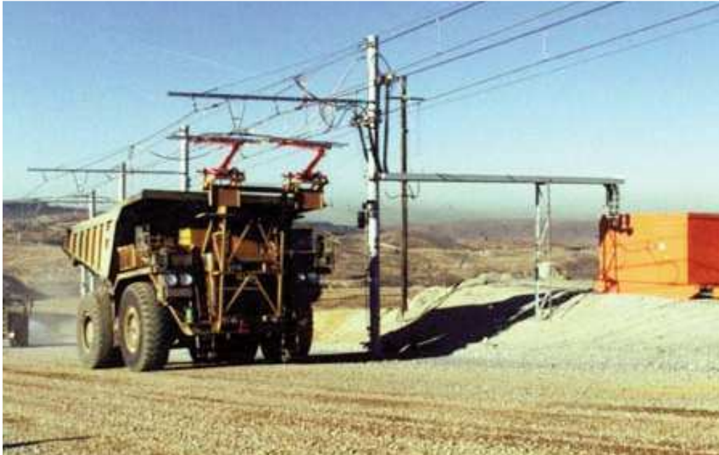
Electric Trolley Assist for Mine Haul Trucks
