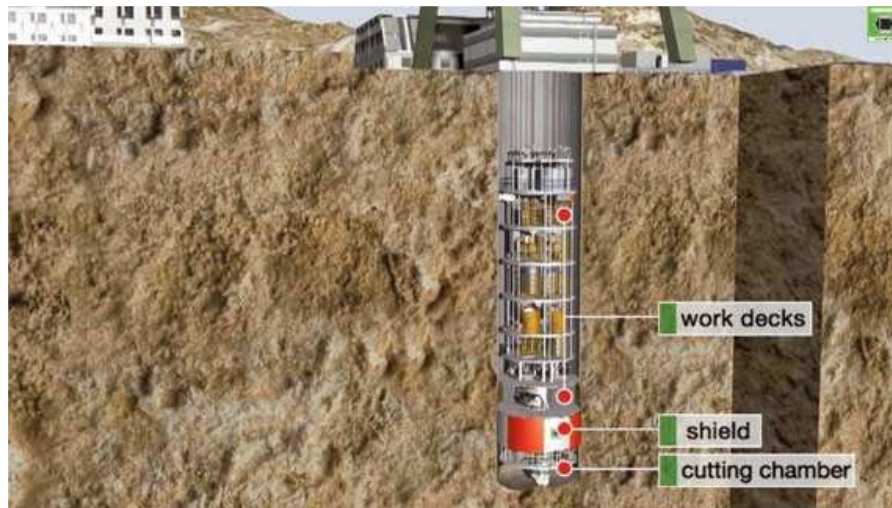
Cross Section of the Herrenknecht Shaft Sinker
